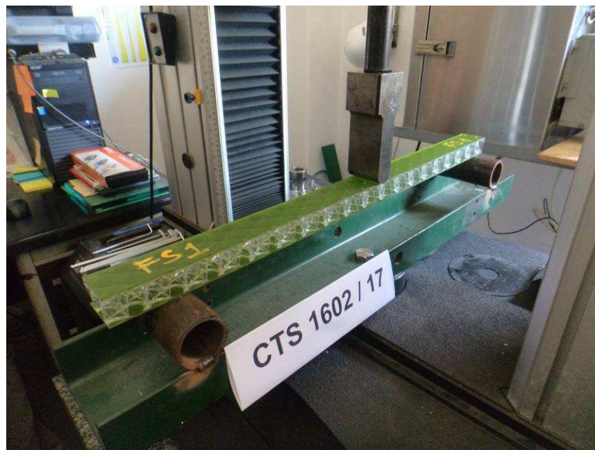
Fig. 3 – Typical arrangement for bending test (UNI EN 310).
