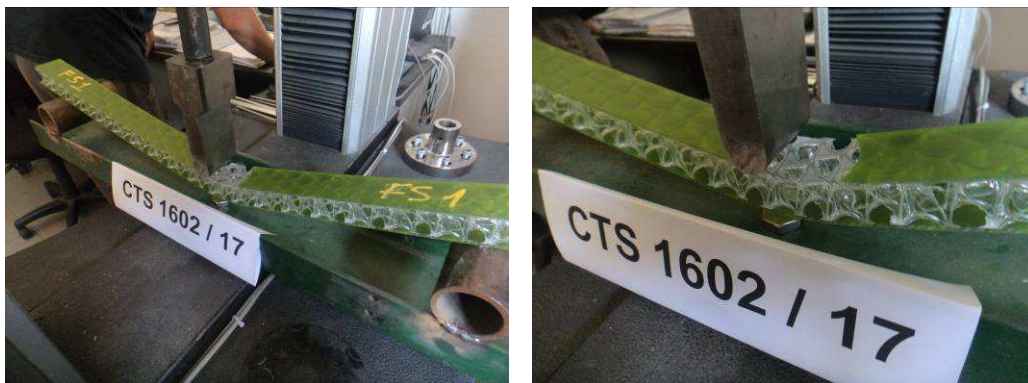
Figs. 5 – 6 Typical specimen failure happened on external layer of composite panel [Specimen FS1].
