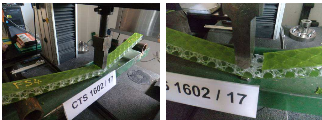
Figs. 7 – 8 Typical specimen failure happened on external layer of composite panel [Specimen FS4].
