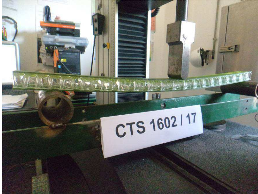
Fig. 4 – Typical arrangement for bending test (UNI EN 310) – Lateral view.
