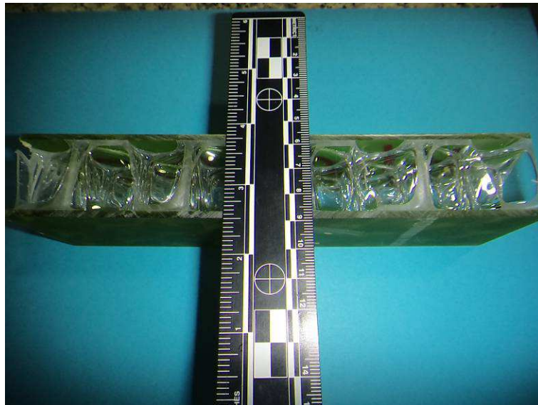
Fig. 2 – View of a sample of composite material through the thickness (34 mm).
